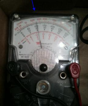
LEADS FROM BATTERY BOX TIED TOGETHER, SWITCH ON TO TEST LIGHT. THE LIGHT WILL ILLUMINATE GRADUALLY AS THE CONDUCTIVITY OF THE WATER INCREASES AS THE COLLOIDAL SILVER STRENGTH INCREASES. THE METER SHOULD BE MONITORED. IN THIS CASE WHEN IT PEGS ON THE .6 MA SCALE I RAISE IT TO THE NEXT SCALE WHICH IS 6 MA. I TOP IT OUT AT 1.2 TO 2.5 MA I MAKE IT STRONGER FOR TOPICAL SKIN USE AND ABOUT 1-1.5 MA FOR INTERNAL AND ORAL USE
